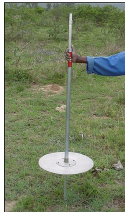
Figure 4: The Disc Pasture Meter (DPM) used for estimating grass fuel loads in the sample plots.
